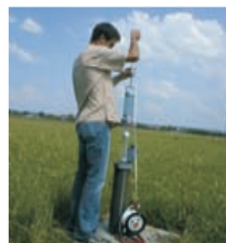
Ground water sampling
